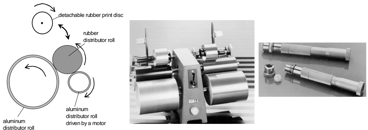
Fig. 10.2.a: Design and photograph of an IGT ink distributor and a photograph of an IGT Ink pipette
