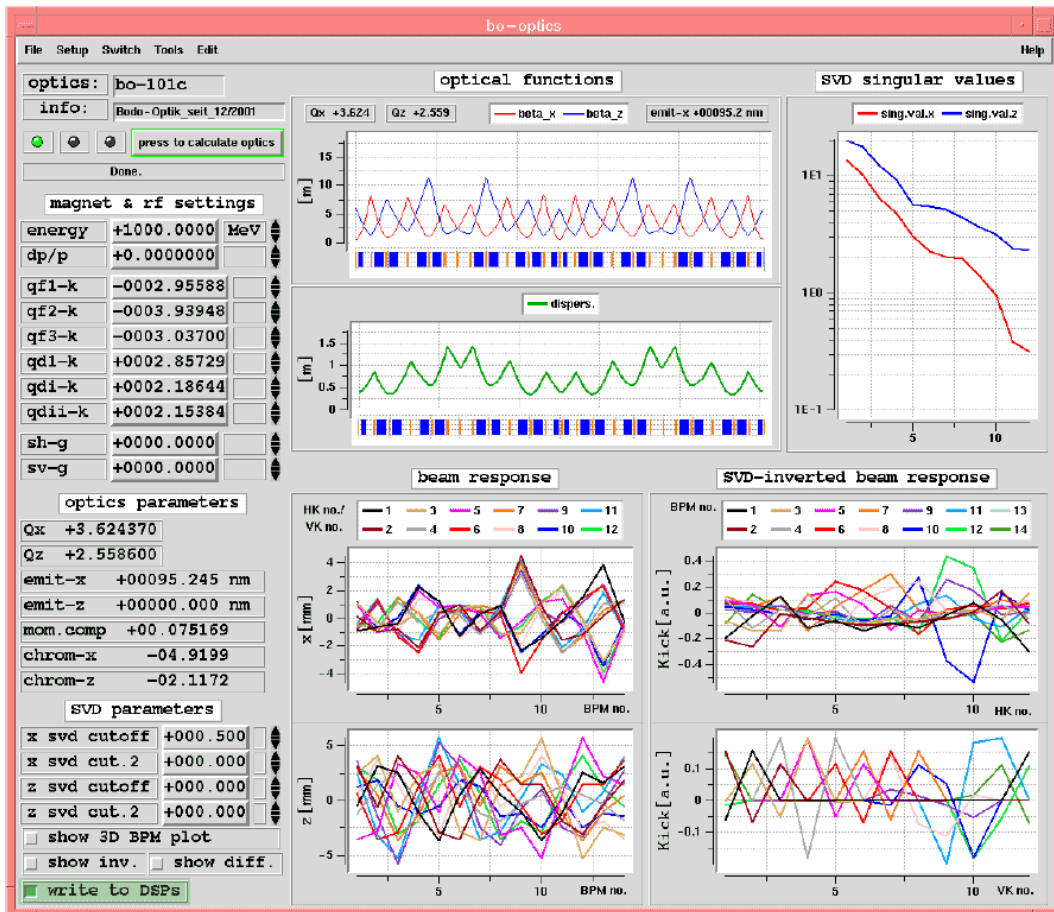
Figure 7.8: Graphical user interface for the online calculation of the Bodo beam optics, of the vertical and horizontal beam response matrices and of the SVD-inverted beam response matrices for the orbit feedback system.
