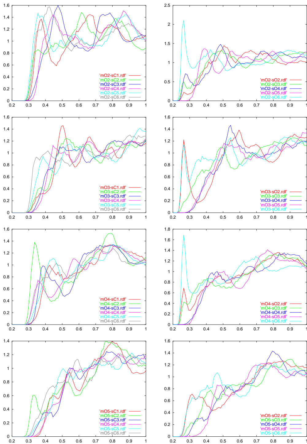
Figure B.3: Part III. Radial distribution functions ( x -axis: r , y -axis: g(r) ) between oligomer and surface atom sites for the (carboxy methyl)cellulose 110-surface simulation. The key shows the respective atoms: the prefix 'm' denotes the oligomer atom type and 's' the surface atom type. Due to the normalization of all rdf to the total number of sites for all oligomers, the limit of g(r) at r \rightarrow \infty depends on the number of adsorbed polyelectrolyte oligomers.
