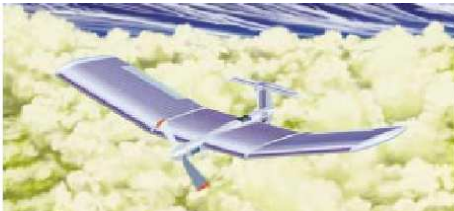
Fig. 3.8: An artists representation of a small unmanned PV powered aircraft that can be used for special missions (e.g. locust spraying in agriculture)
