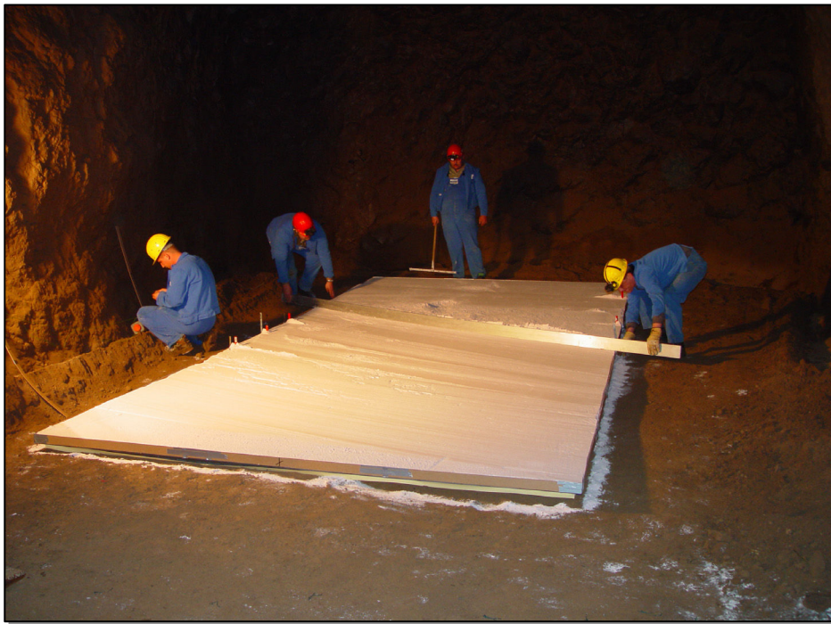
Figure 6: Preparation of a plate sandwich for cladding in the underground mine DYNAenergetics uses. The ANFO explosive is homogenously distributed with an Aluminium lath to guarantee a homogenous layer thickness.
