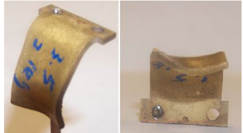
Non uniform flanging of 1.588mm specimen
