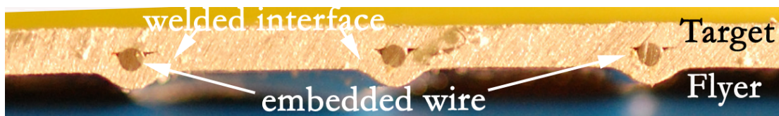
(c) Welded sample with embedded wires
