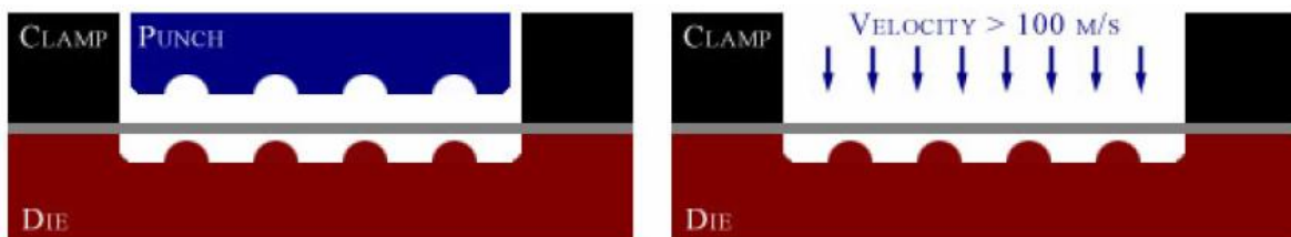
Figure 1: Schematic illustrations of conventional stamping (left) and electromagnetic forming (right) [4]
