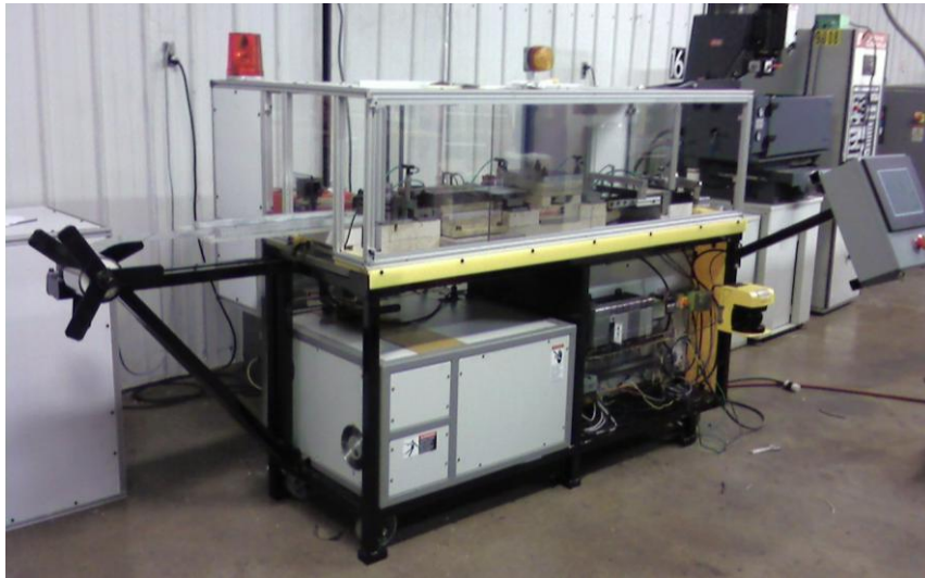
Figure 4: Prototype machine for bipolar plate manufacturing by compliant layer electromagnetic forming
