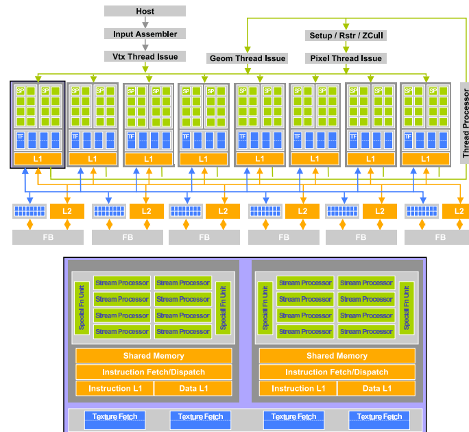
Figure 3.3: NVIDIA GeForce 8800 GTX block diagram. Image courtesy Owens et al. [176].
