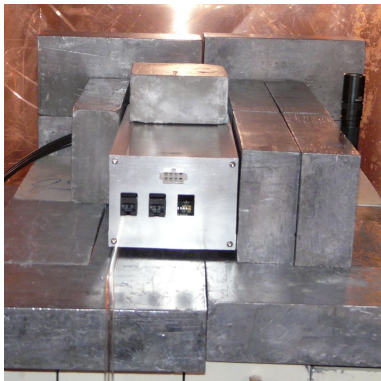
Figure 3.3: The polaris pixel detector setup at LNGS during construction.
