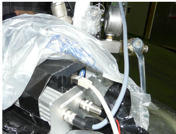
Figure 2.10: The liquid nitrogen Dewar with the monitoring and control electronics box.
