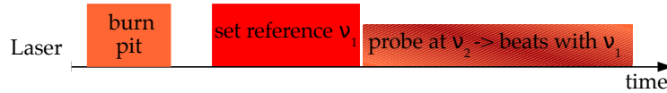
Figure 11: Coherence beat experiment pulse sequence. Using chirped pulses a transparent window (pit) is prepared in the inhomogeneously broadened optical line. The optical reference coherence is excited with a laser pulse of frequency \nu_1 , outside the pit. The probe field has a frequency of \nu_2 = \nu_1 + 13 MHz and is in the centre of the transparent pit.
