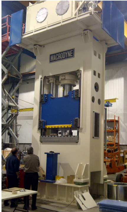
900 ton warm/hot forming press
