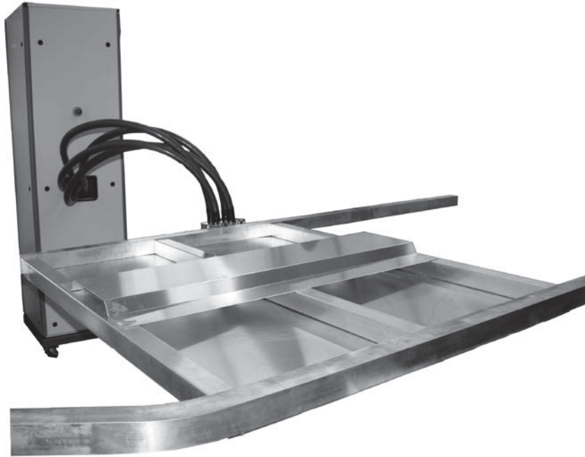
Figure 6: EMPT welding of larger subassemblies
