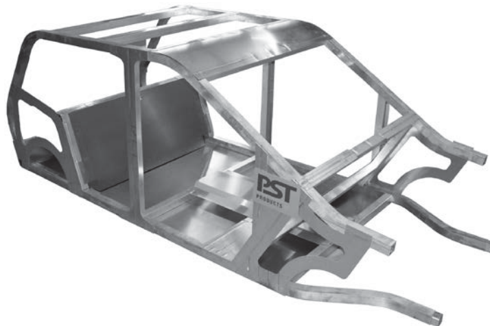
Figure 7: EMPT welded space frame
