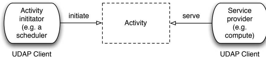
Figure 5.2.: An activity as an intermediary between an activity owner/initiator and a service provider serving that activity. The box labelled 'Activity' represents the abstract activity entity (cf. also Figure 5.1).
