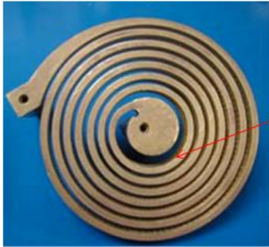
Deformed central turn with increased clearance between the 1st and 2nd turns
