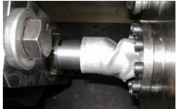
Figure 15: Failure mode 2: tube buckling, without cracking
