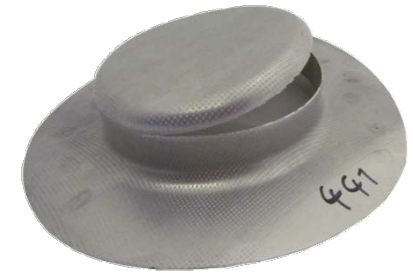
Bottom tear at a cylindrical cup
