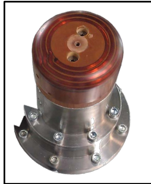
Punch with integrated coil turns
