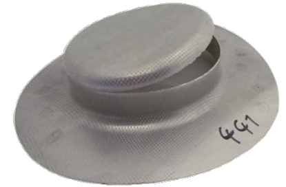
Bottom tear at a cylindrical cup
