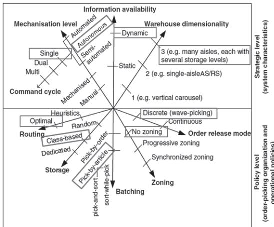
Figure 4-20: Design and Operational Parameters of the Order-picking and Storage System of the CTS based on (De Koster, et al., 2007)
