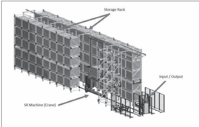
Figure 2-3: AS/RS and its components
