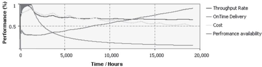
Figure 5.18: Performance availability calculated based on the weighted average method.
