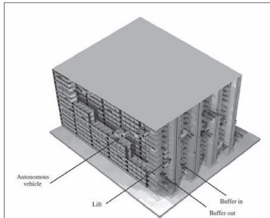
Figure 2-4: AVS/RS and its components (Marchet, et al., 2012).
