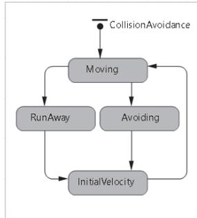
Figure 4-9: Collision Avoidance State Chart.
