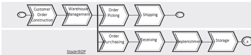
Figure 4-3: The main processes of the Cellular Transport System
