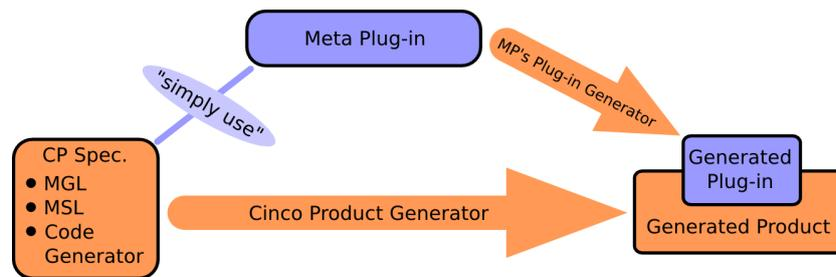
Fig. 3.2: Meta plug-ins contribute to the CInco product generator and provide a generative way of service orientation.
