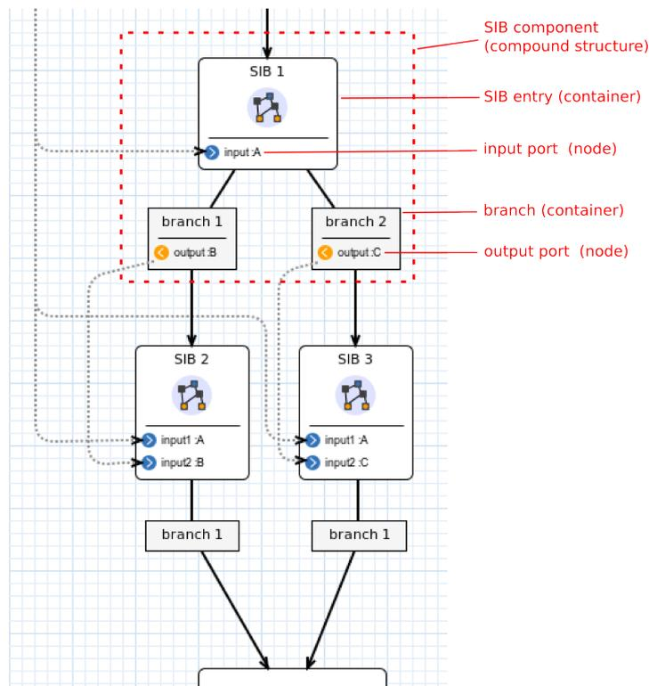
Fig. 6.1: A DIME SIB component comprises of various CInco containers and nodes.
