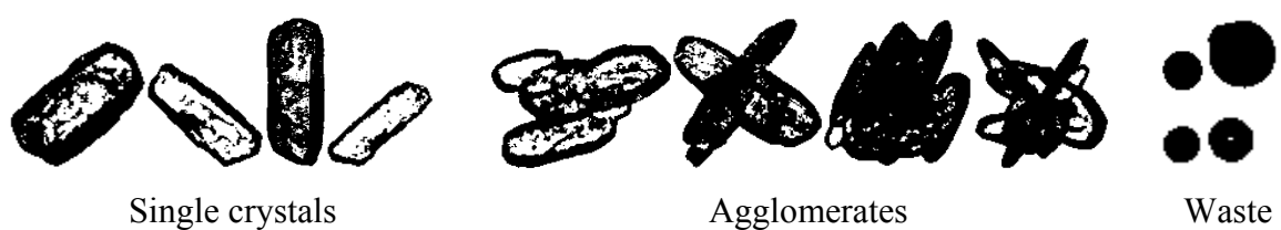
Figure A.10: Images of single crystals, agglomerates, and waste particles recorded with the QICPIC for the material system adipic acid/ water [119]
