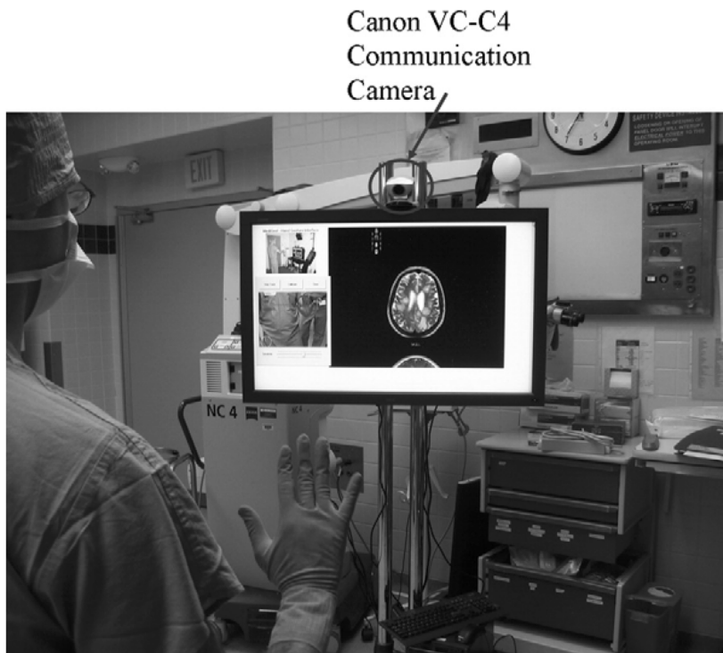
Figure 2.12: Hand gesture interface for medical visualization applications (Gestix). The image is adopted from Wachs et al. (2008). ©2008 IEEE
