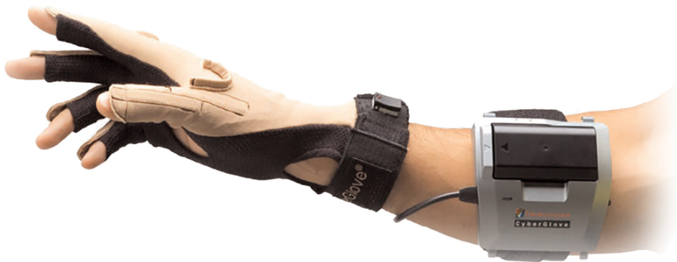
Figure 2.1: CyberGlove sensor (CyberGlove Systems LLC, 2017) as an example of contact based technology. ©2017 CyberGlove Systems LLC.
