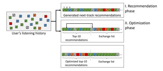
Figure 2.5: Illustration of the re-ranking scheme, adapted from [Jug+17].
