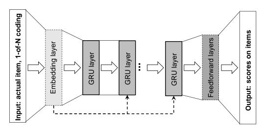
Figure 2.2: General architecture of the GRU-based RNN model, adapted from [Hid+15].
