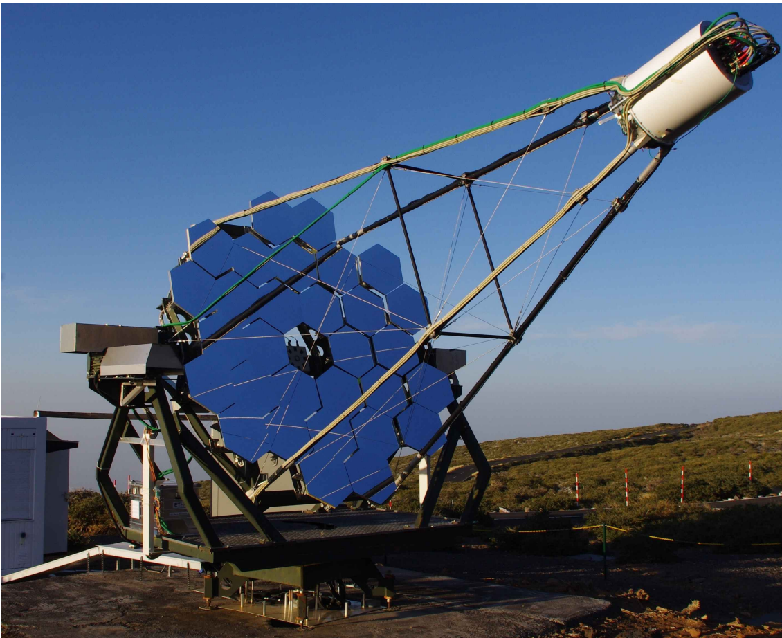
Figure 3.5: Photograph of the FACT telescope. The single hexagonal mirrors forming the primary mirror can be seen as well as the camera (white cylinder) in the top right. The image is taken from [Aea13].
