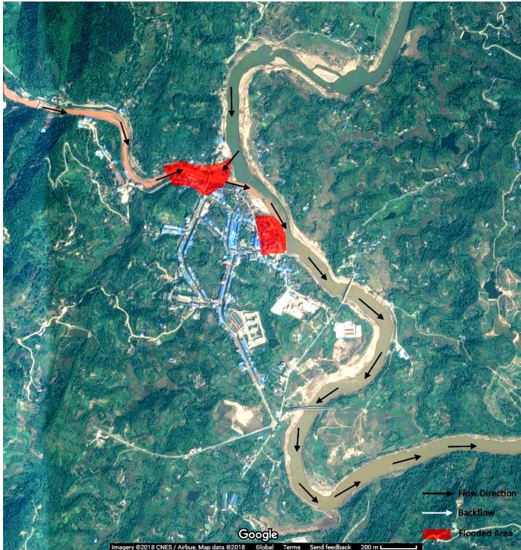
Figure 8.11 Illustration of river flow direction and the backflow flood affected area in Tongjing Town.
