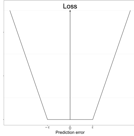
Figure 7.8.: \epsilon -insensitive loss function for SVR. Prediction errors with deviation less than \epsilon will not be penalized. A deviation above will be penalized linearly dependent on the parameter C
