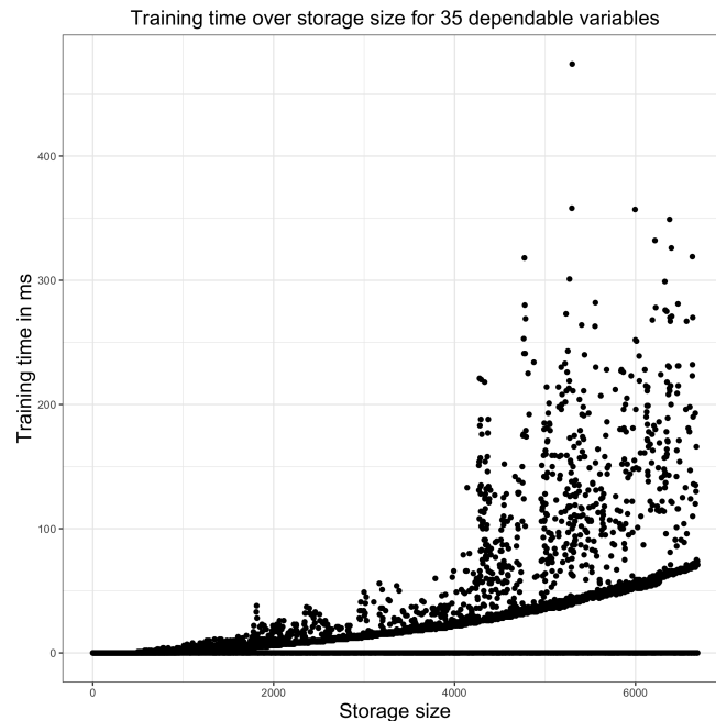
Figure 7.10.: Training time in ms over sample size for incremental SVR. The storage size is assumed to be indefinite and no sample was removed.
