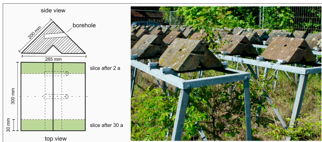
Figure 1. Left: The geometry of the samples and the sampling of the sample slices after 2 and 30 years, here marked green (years = a). Right: Outdoor weathering of the samples in Nuremberg after an exposure time of 30 years.
