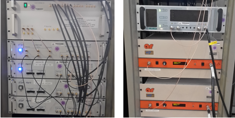
Figure 3.5.: Photo of the bunch-by-bunch feedback system units and the corresponding amplifiers at DELTA. Left: From top to bottom, the clock and trigger unit, the combined front-/backend unit and the three FPGA-based gigasample-processors. Right: The three amplifiers (longitudinal at the top, transverse below) send the output signals of the feedback system to fast-pulsed kicker structures.
