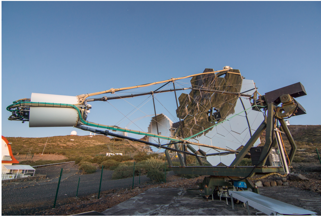
Figure 2.1: FACT in front of the MAGIC-II telescope at the Observatorio del Roque de los Muchachos. The white cylinder on the left is the camera, complete with all readout electronics.
