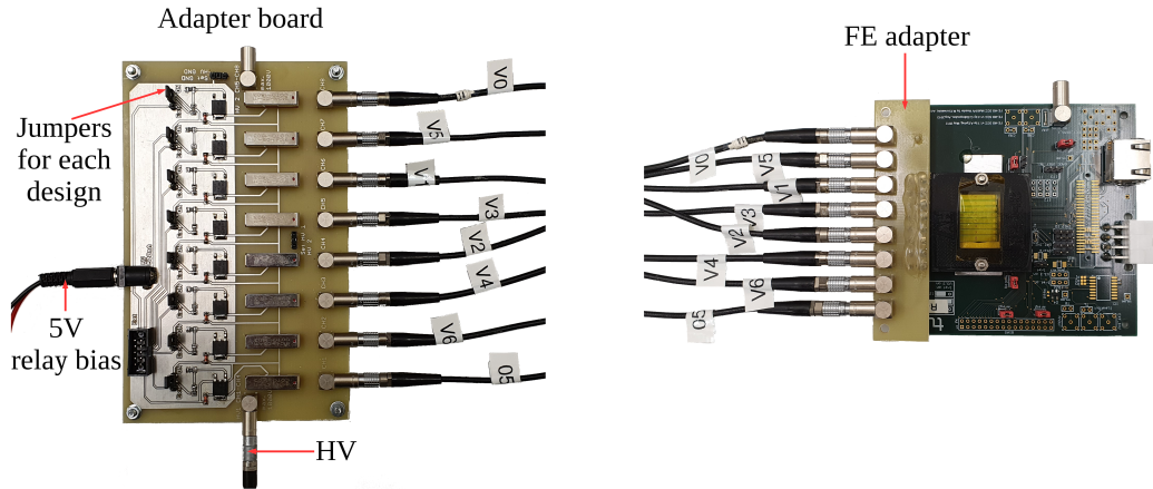
Figure 6.3: Image of the adapter board and FE adapter to bias selected individual pixel designs from outside the measurement setup. 5 V biased relays controlled with jumpers distribute the HV to the selected pixel design groups.
