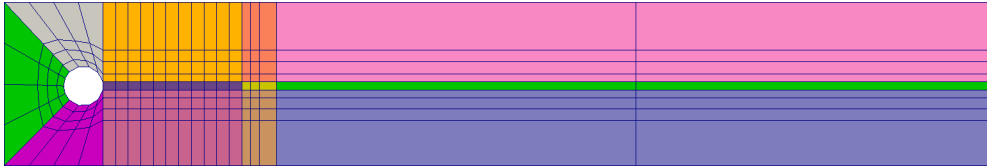
Figure 5.12: Multi-patch NURBS mesh (coarsest level) used for FSI tests 1-3. The elastic bar is resolved with 11 elements along the x-axis.
