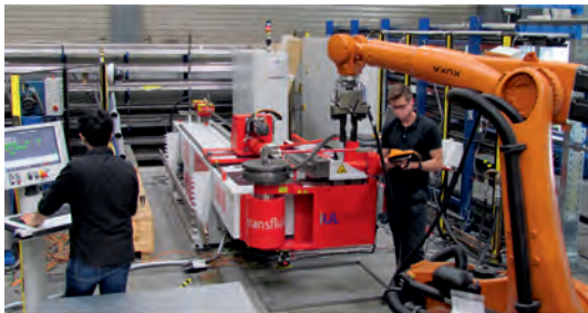
Installation of the new tele-operative bending cell
