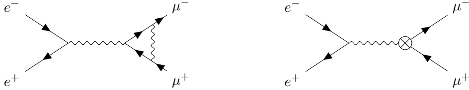
Figure D.1: Virtual corrections to the tree level process of e^- e^+ \rightarrow \mu^- \mu^+ scattering at NLO in the muon coupling.
