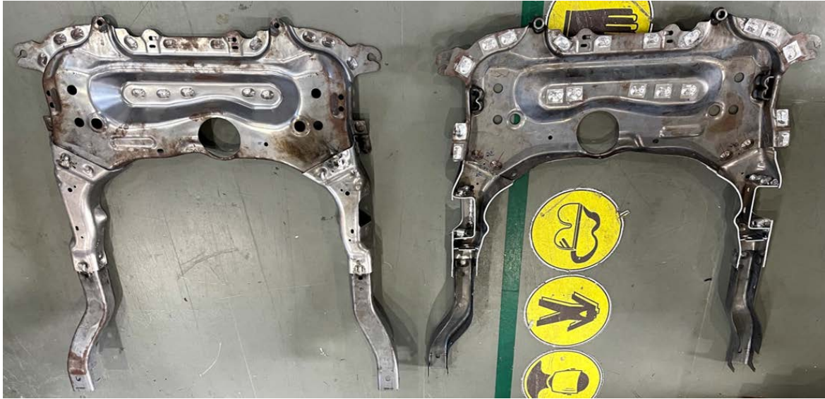
Figure 5: Two VFA welded prototype subframes (in progress).
