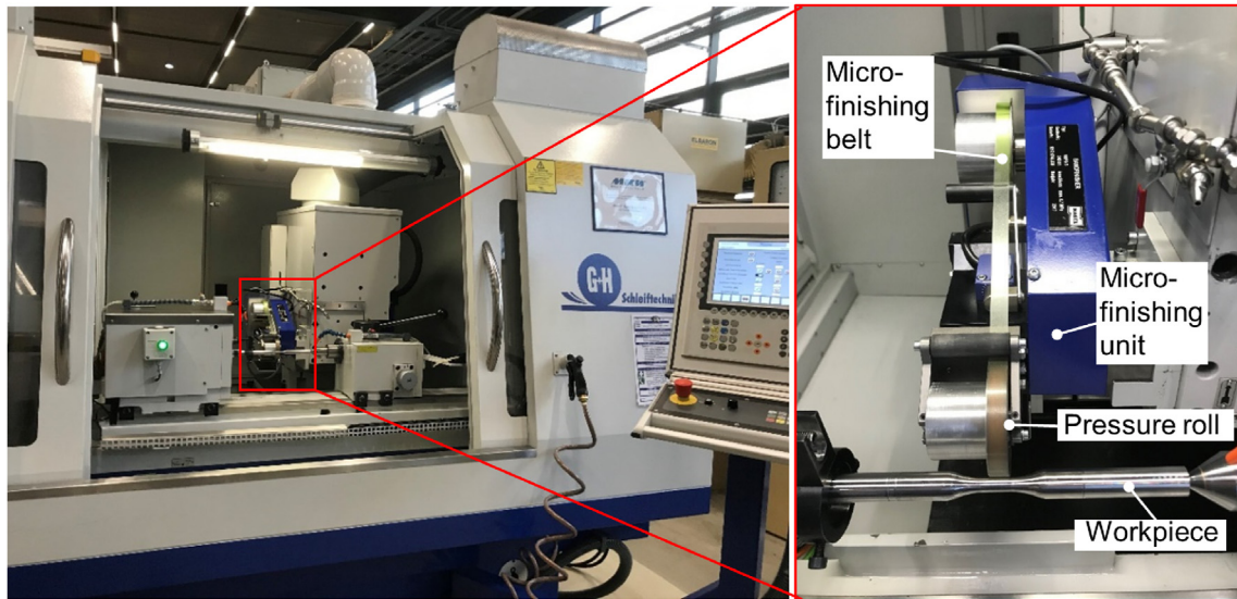
Fig. 3 – Experimental setup for microfinishing of the two types of specimens.
