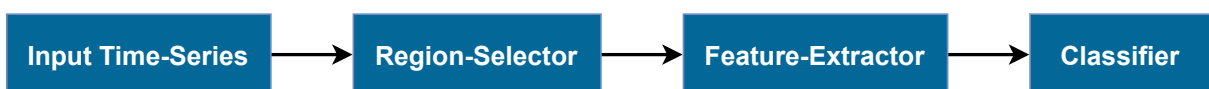
Figure 4.10: Basic architecture of traditional object detection algorithms based on Xiao et al. (2020)
