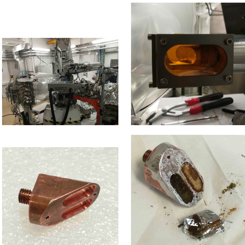
Figure K.1: Exploratory XRS measurements at the GALAXIES beamline at the SOLEIL synchrotron, France. Top left: The combined setup for detection of both XES and XRS signals by use of a Johann type spectrometer and a dispersive von Hamos type spectrometers. Top right: Sample environment; Sample holder and cryostat cap, installed. Bottom right: Detail view of the canted sample holder for reflection geometry simultaneous XES and XRS measurements. Bottom right: Samples after the measurements. In this case, clear signs of radiation induced changes in the sample are visible.
