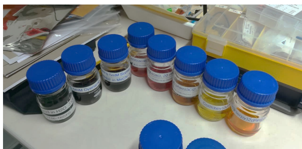
Figure 2.1: A selection of cobalt-based TM complexes in solution. The wide range of observed colors arises due to the properties of the valence electrons, which are, as many chemical properties in these compounds, dictated by the intricacies of the metal d-orbitals and the nature of the ligands (see text).
