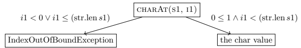
Figure 4.5: The thrown exceptions for the CHARAT method depending on the numeric constraints involved.
