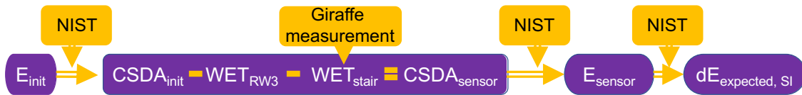
Figure 7.2: Calculation of the expected deposited energy in 200 \mu\text{m} silicon dE_{\text{expected,SI}} using the NIST database, the WET of the RW3 plates, and the WET of the corresponding ROI for the staircase phantom. [20]
