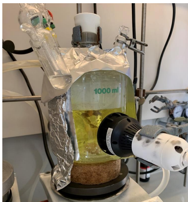
Figure 4.7. Reaction setup for the photosensitized [2+2] cycloaddition.
