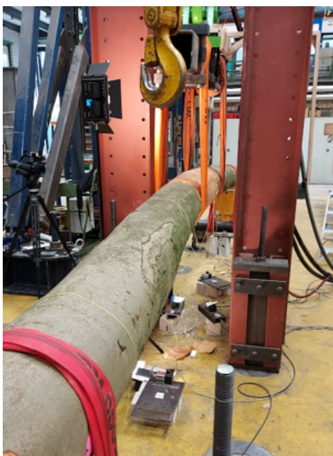
(a) Shaft of 6m length in the bending test installation
