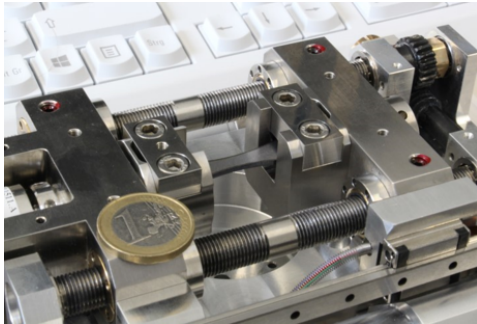
(a) Micro-testing machine by Kammrath & Weiss GmbH.
